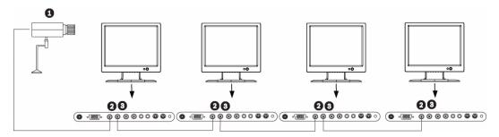
Figure 6.6 Multiple Monitor Configuration
