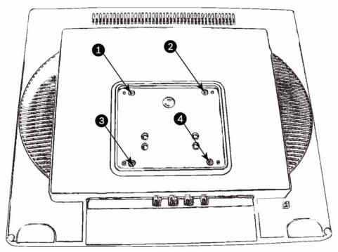
Figure 6.2 Mounting the Device
